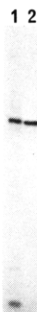
Figure 2. Analysis of 32 P-labeled oligonucleotides by polyacrylamide (20%) gel electrophoresis in 7 M urea. Lane 1 represents the crude oligonucleotide mixture containing the 29-mer (5'-AATTCACATACCTCTTTCCCTCTCTGCT). Lane 2 shows the same 29-mer after HPLC purification.
